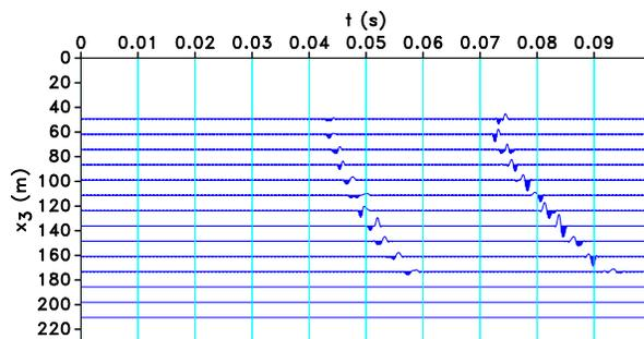
Figure 7: Vertical component of the recorded displacement after windowing of the direct P- and SV-waves.
