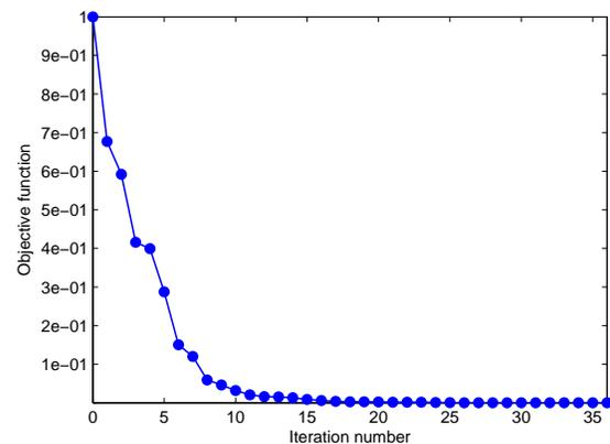
Figure 2: Change of the normalized objective function  $\mathcal{F}(\mathbf{m})$  with iterations for the model in Figure 1. Parameter updating was carried out with the NCG method. The origin time  $t_0$  is fixed at the correct value.
