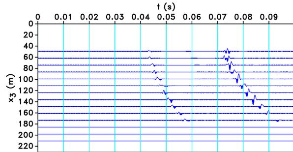
Figure 8: Difference between the recorded vertical displacement (Figure 7) and the displacement computed for the initial model. The scale is the same as in Figure 7.
