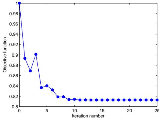
Figure 4: Change of the normalized objective function  $\mathcal{F}(\mathbf{m})$  with iterations for the model in Figure 1. The inversion was performed on noise-contaminated data (see Figure 3).
