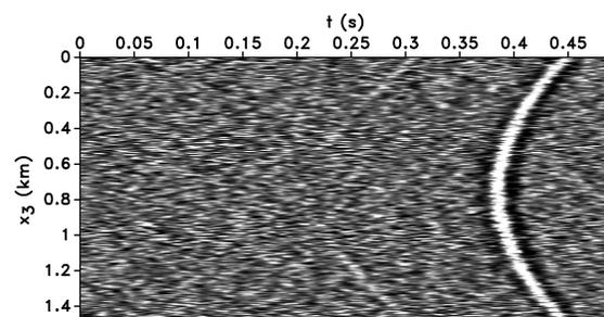
Figure 3: Vertical displacement of the observed data contaminated with Gaussian noise for the model in Figure 1. The noise has the same frequency band as the data with the variance equal to 0.07% of the maximum amplitude.
