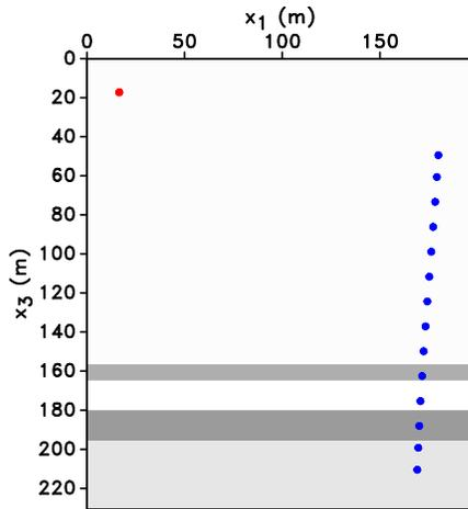
Figure 6: Acquisition geometry for the microseismic survey at Bakken field. Microseismic event (red dot) and a tilted array of receivers (blue dots) are embedded in a layered VTI medium. The average spacing between the receivers is 12.4 m. The interval medium parameters are listed in Table 1. The initial source location is  $x_1 = 16.52$  m,  $x_3 = 17.29$  m.
