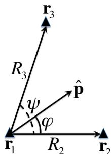
**Figure 1.** The location of the stations at  $\mathbf{r}_1$ ,  $\mathbf{r}_2$  and  $\mathbf{r}_3$ , the definition of the interstation vectors  $\mathbf{R}_2$  and  $\mathbf{R}_3$ , the angle  $\psi$  between these vectors, and the polarization vector  $\hat{\mathbf{p}}$  at azimuth  $\varphi$ .
