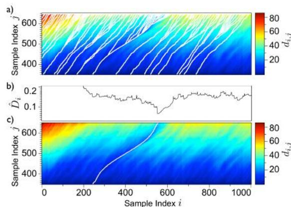
**Figure 8.** Paths backtracked (a) from every sample in the top row overlaid on the array of distances. Values in the normalized top row of the array of distances  $\hat{D}_i$  (b) have a clear minimum. The optimal warping path (c) corresponds to the smallest value of  $\hat{D}_i$  and follows valleys of distances.
