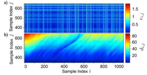
**Figure 6.** The array of squared alignment errors (a) for the two sequences in Figure 5. The array of distances (b) is defined by equations 6 and 7. A path with small alignment errors is apparent between sample indices of  $i = 250$  and  $i = 550$ .
