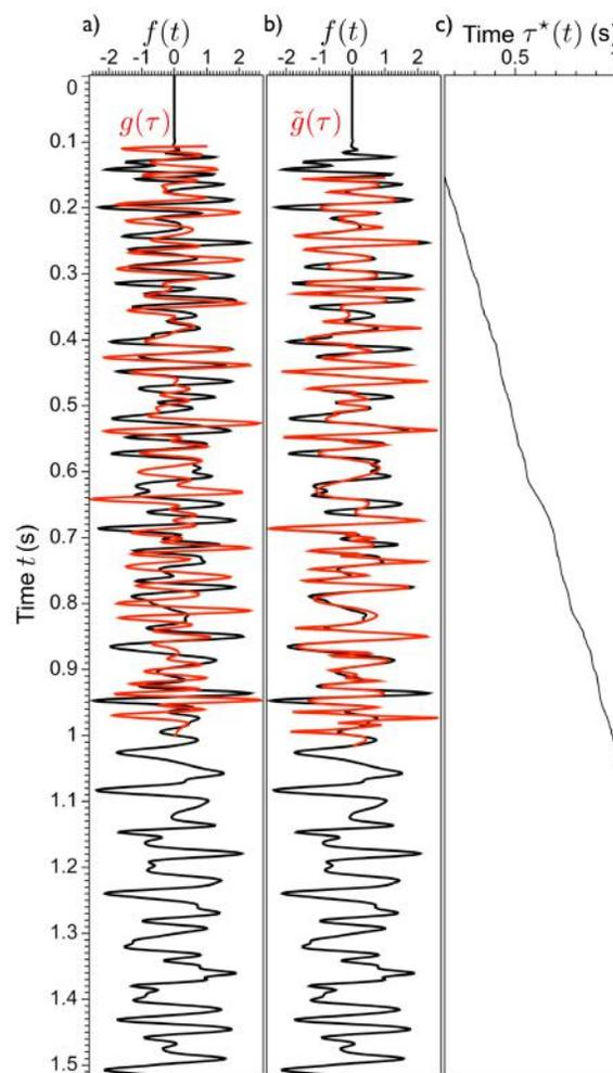
**Figure 12.** The original synthetic  $g(\tau)$  (a) is overlaid on a portion of the seismic trace  $f(t)$ . The warped synthetic  $\tilde{g}(\tau)$  (b) has an 84 degree phase rotation.  $\tau^*(t)$  (c) is the function used to warp the synthetic seismogram.
