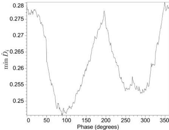
**Figure 13.** The minimum value of  $\hat{D}_i$  (a) varies with a constant phase rotation applied to the synthetic seismogram. We choose the phase to be 84 degrees, because that constant phase rotation yields the smallest value of  $\min \hat{D}_i$ .
