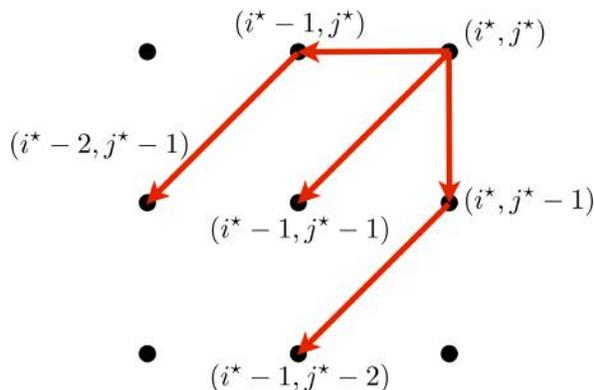
**Figure 7.** A schematic of the potential warping paths from  $(i^*, j^*)$  in the backtracking procedure. Black dots represent samples in the array of distances, while red arrows are potential additions to the warping path.
