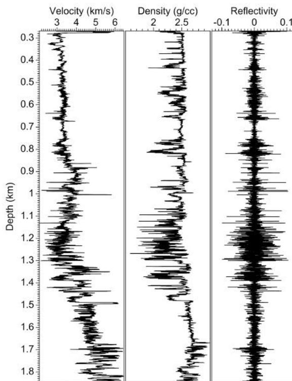
**Figure 2.** Teapot Dome well UWI 490252305400 has a P-wave velocity log and density log. Acoustic reflectivity in the rightmost panel is computed using equation 1.
