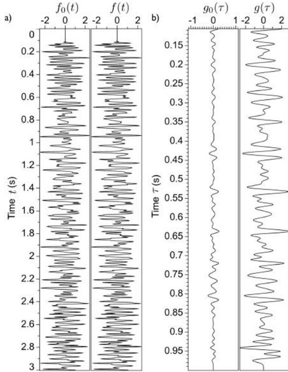
**Figure 4.** The difference between the seismic trace before and after ( $f_0(t)$  and  $f(t)$ ) normalization (a) is negligible. The difference between the synthetic seismogram before and after ( $g_0(\tau)$  and  $g(\tau)$ ) normalization (b) is significant.
