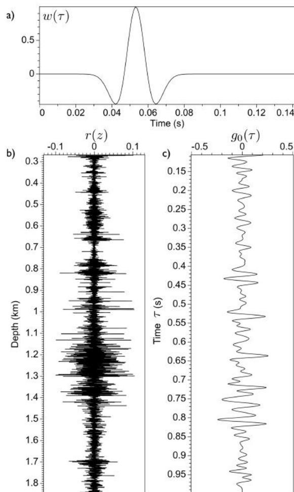
**Figure 3.** The wavelet  $w(\tau)$  (a) is a constant Ricker wavelet with a peak frequency of 35 Hz. The reflectivity  $r(z)$  (b) is computed using equation 1. The synthetic seismogram  $g_0(\tau)$  (c) is computed using equation 3.
