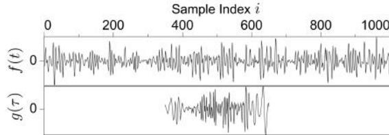
**Figure 5.** Artificial sequences used to illustrate DTW, where the sequence  $g(\tau)$  is a warped and bulk shifted segment of the sequence  $f(t)$ .
