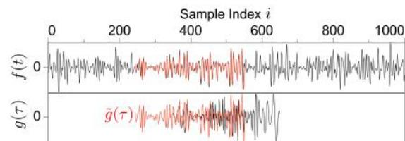
**Figure 9.** The artificial sequences as shown in Figure 5.  $g(\tau)$  is a warped and shifted segment of  $f(t)$ . Using the DTW optimal warping path (Figure 8c),  $g(\tau)$  is corrected to  $\tilde{g}(\tau)$ .
