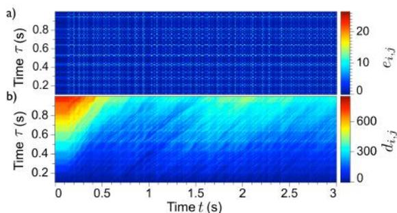
**Figure 10.** The array of squared alignment errors (a) and distances (b) for the Teapot Dome data. Times  $t$  correspond to the seismic trace, and times  $\tau$  correspond to the synthetic.
