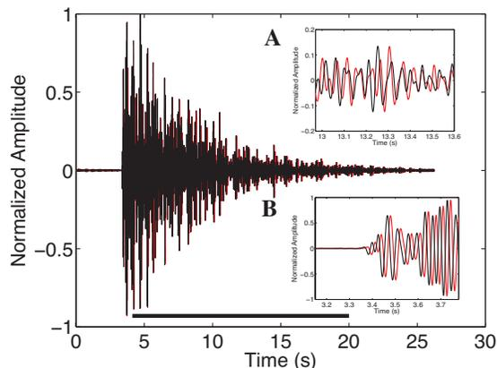
**Figure 3.** Recorded seismic signals at station E (Figure 2), the reference signal (red line) and the recorded signal (black line) with 0.4% relative velocity change. Inset A shows the late coda while inset B shows the first arrivals of the two signals. The black bold line is the time window used for data processing.
