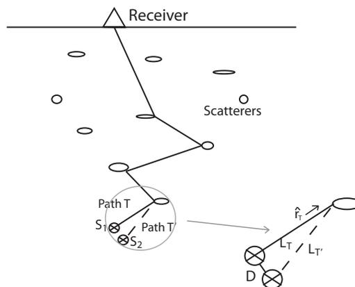
**Figure 1.** Geometry of wave paths. Source,  $S_1$ , produces the unperturbed signal while Source,  $S_2$ , produces the perturbed signal. Path  $T$  shows the scattering path for the unperturbed signal and the scattering path for the perturbed signal is defined by Path  $T'$ . The sources are separated by a distance  $D$  and the source distances are  $L_T$  and  $L_{T'}$  distance away from the first scatterer along path  $T$  and  $T'$ , respectively.
