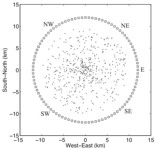
**Figure 2.** The experiment geometry of the numerical simulation. The receivers (squares) are surrounding the point scatterers (black dots). The source is positioned in the origin (cross). All perturbations of the source location is done from this position. The stations marked (NW, NE, E, SE, and SW) are used in the presentation of results in Figures 7 and 8.
