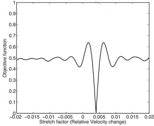
**Figure 4.** The objective function  $R(\epsilon)$  as a function of the stretch factor  $\epsilon$ . The objective function is minimum for  $\epsilon = 0.4\%$ , which corresponds to the time velocity change.
