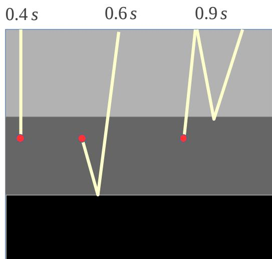
**Figure 15.** Sketch of some events that are present in the Green's function from the virtual source (red dot) at 1000m and recorded at the surface.
