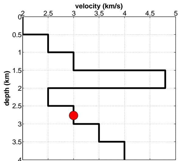
**Figure 4.** Velocity model with high impedance layer at 1.5 km; the dot is the position of the virtual source.
