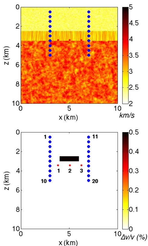
**Figure 9.** Numerical model for time-lapse localized velocity change. The reference velocity (scattering) model (a) with the source-receiver setup, and the exact localized velocity change (b) with the source-receiver setup.
