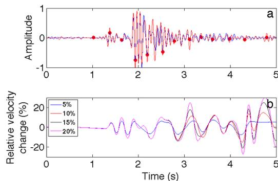
**Figure 8.** Relative velocity changes (b) computed from the 5-15Hz bandpassed time-lapse microseismic signals (a) using SDTW and multiple bounds on  $du/dt$ . Time shifts are sampled on an amplitude-aligned coarse grid (red points) (a).
