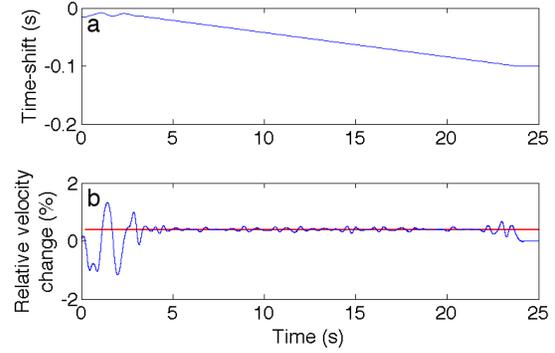
**Figure 4.** Time shifts and relative velocity changes estimated via SDTW. The time shifts (a) and the relative velocity changes (b) are computed from the synthetic time-lapse signals shown in Figure 1. We compare the exact velocity change (red) to the estimated relative velocity changes (blue) (b).
