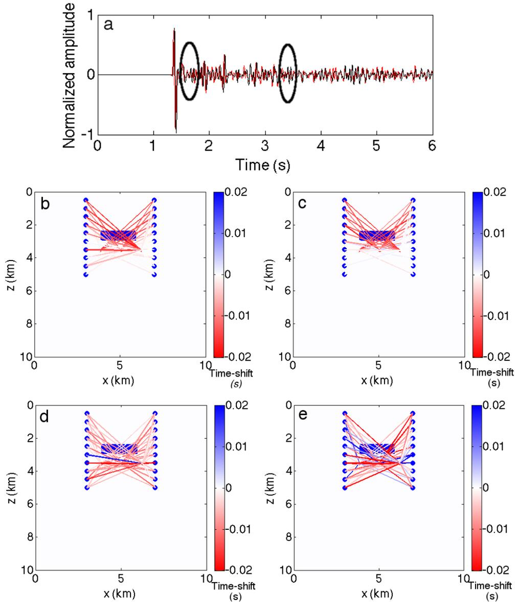
**Figure 11.** The early (near  $t = 1.6$  s) and late (near  $t = 3.4$  s) coda of the time-lapse signals (a) are highlighted. Time shifts from the early coda are computed using the stretching method (b) and SDTW (c), and time shifts in the late coda are also computed using the stretching method (d) and SDTW (e). The colored lines indicate the magnitude of the estimated traveltime changes.
