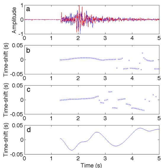
**Figure 5.** Time shifts computed from the unfiltered time-lapse microseismic signals (a) using windowed cross-correlation (b), the windowed stretching method (c), and SDTW (d).
