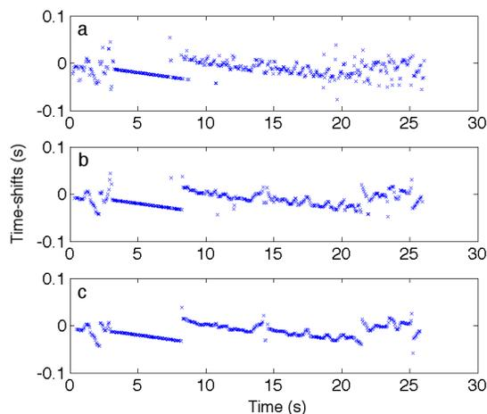
**Figure 2.** The stability of the windowed cross-correlation method for time shift estimation. The time shifts are estimated within time windows whose widths are relative to the dominant period  $T$  of the signal:  $2t_w = 37.5T$  (a),  $2t_w = 75T$  (b), and  $2t_w = 112.5T$  (c), where  $T = 0.033$  s.
