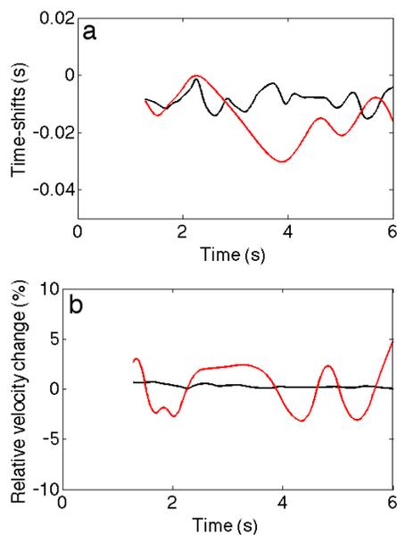
**Figure 10.** A comparison of the estimated time shifts (a) and relative velocity changes (b) using stretching method (black) and smooth dynamic warping (red). These timeshifts and velocity changes are estimated using the time-lapse signals for Source 2 and Receiver 3 pair shown in Figure 9.
