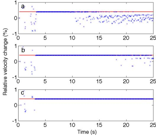
**Figure 3.** The stability of the windowed stretching method for relative velocity change estimation. The relative velocity changes are estimated within time windows whose widths are relative to the dominant period  $T$  of the signal:  $37.5T$  (a),  $75T$  (b), and  $112.5T$  (c), where  $T = 0.033$  s. The red line shows the exact relative velocity change.
