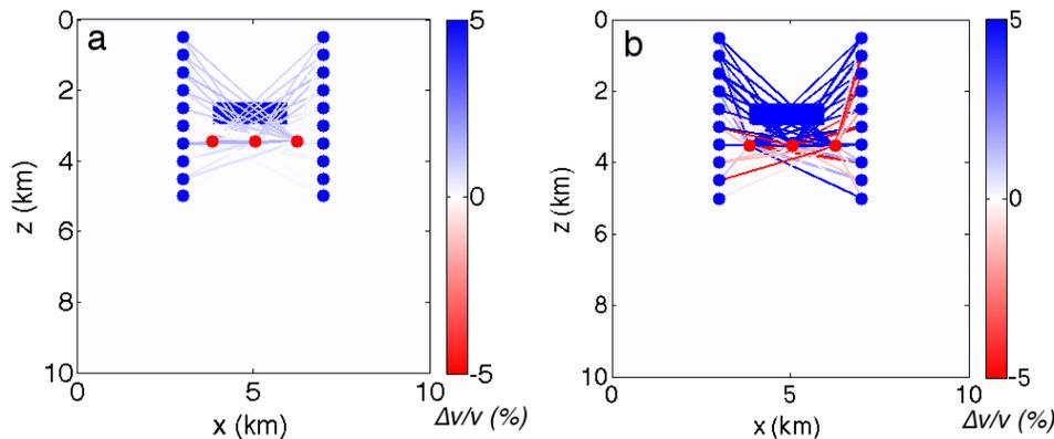
**Figure 12.** Distribution of the relative velocity changes between time-lapse signals computed using the stretching method (a) and SDTW (b) among source-receiver pairs. The velocity changes are estimated using the early part of the time-lapse coda. Blue circles are the receivers while the red circles are the sources. The blue rectangle gives the localized time-lapse velocity change of 5%. The colored lines indicate the magnitude of the estimated relative velocity changes.
