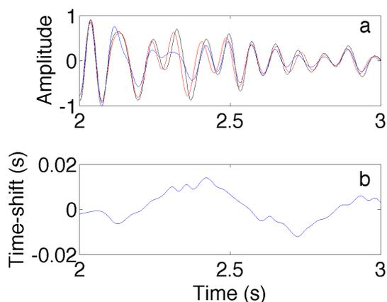
**Figure 7.** The 5-15Hz bandpassed time-lapse microseismic baseline signal (a) (blue), time-lapse signal (a) (red), and aligned time-lapse signal (a) (black). The time shifts (b) used to align the time-lapse signal to the baseline signal are computed using SDTW.
