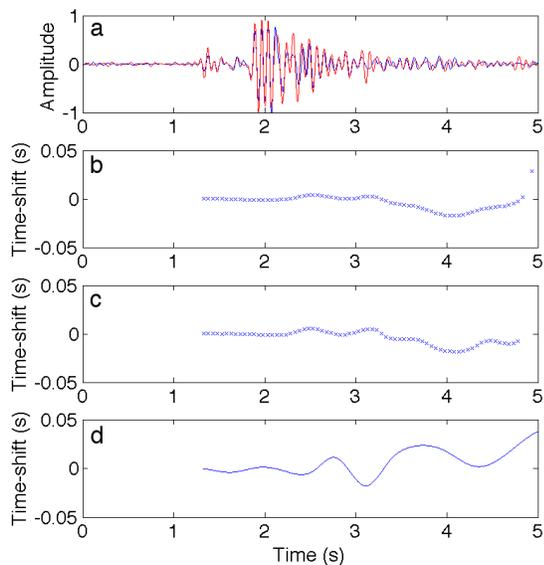
**Figure 6.** Time shifts computed from the 5-15Hz band-passed time-lapse microseismic signals (a) using windowed cross-correlation (b), the windowed stretching method (c), and SDTW (d).
