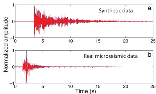
**Figure 1.** Synthetic time-lapse signals (a) and recorded microseismic time lapse signals (b). The blue curve is the baseline signal and the red curve is the time-lapse signal.
