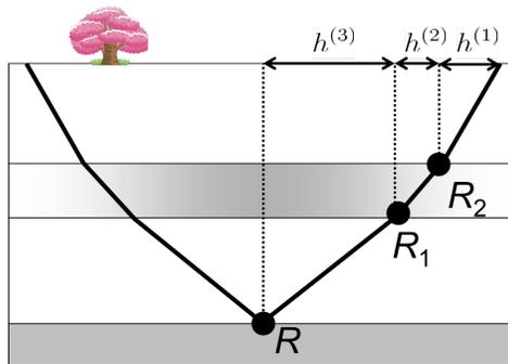
**Figure 1.** Reflection raypath through a horizontal three-layer model.  $h = h^{(1)} + h^{(2)} + h^{(3)}$  is the half offset,  $R$  is the reflection point for the unperturbed ray, and  $R_1$  and  $R_2$  are the intersection points with layer boundaries. Following Grechka and Tsvankin (1999), the raypath perturbation caused by weak lateral heterogeneity is assumed to be negligible, and the ray is confined to the vertical plane. Only in the second layer is laterally heterogeneous.
