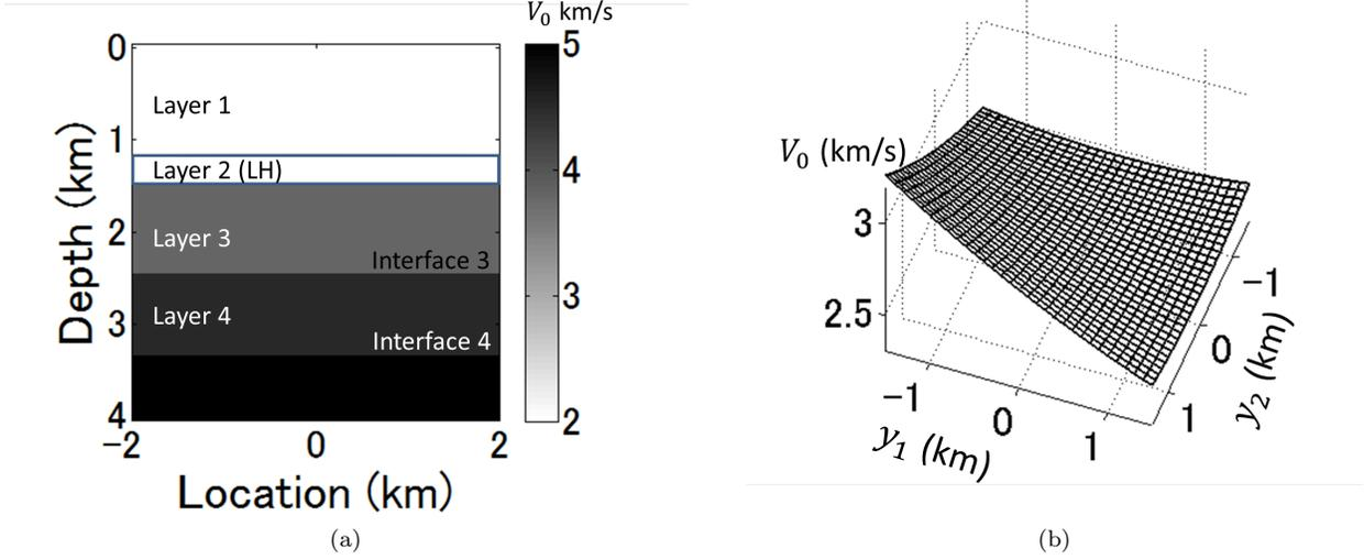
**Figure 5.** (a) Stratified HTI model that includes an isotropic LH layer. (b) Lateral variation of the vertical velocity  $V_0$  in the LH layer.
