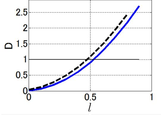
**Figure 2.** Coefficient  $D$  computed from equation 7 as a function of  $l$  for  $k = 0.1$  (solid line) and  $k = 0.2$  (dashed).  $D=1$  (thin horizontal line) corresponds to a single LH layer.
