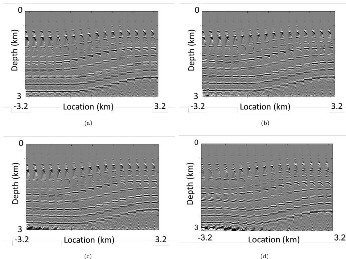
**Figure 8.** Image gathers for the model from Figure 7 computed using (a) actual model parameters; (b) parameters obtained by our MVA algorithm (“full MVA”), (c) parameters obtained by MVA without taking  $k_{x2}$  in the thin layers into account using a block width of 1.5 km; and (d) parameters obtained by MVA in the layer-stripping mode. The estimated parameters of the TTI layers are listed in Table 3. The maximum offset is 4.5 km.
