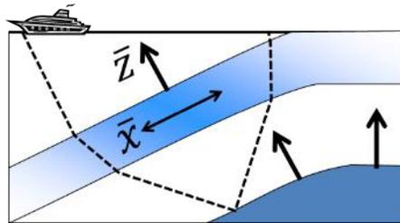
**Figure 2.** Schematic section of a three-layer TTI model. The symmetry-direction velocity  $V_0$  varies as a quadratic function of the distance along the layer boundaries. The symmetry axis of the TTI layer is perpendicular to its bottom.
