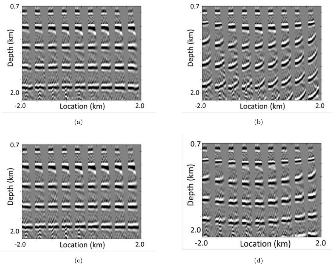
**Figure 5.** Image gathers for the model in Figure 4 obtained with the (a) actual model parameters; (b) laterally homogeneous, isotropic initial model; (c) model estimated by MVA; (d) parameters obtained in the layer-stripping mode with fixed  $k_{x2} = 0$  in layers 2 and 3. The maximum offset is 4 km.
