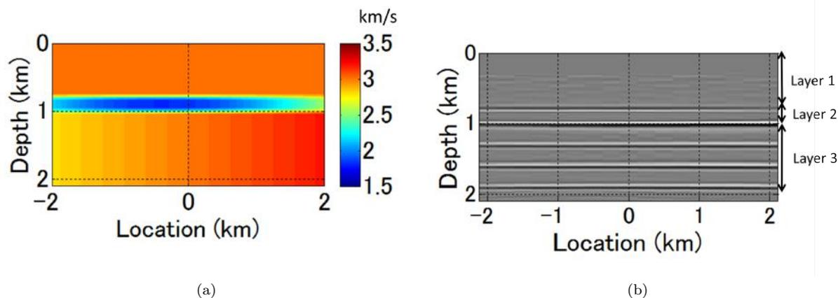
**Figure 4.** (a) Model composed of three horizontal layers with quadratic lateral velocity variation in the middle (second) layer. The top layer (Layer 1) is homogeneous and isotropic with  $V_0 = 3$  km/s. Layer 2 is isotropic with  $V_0 = 1.8$  km/s,  $k_{x1} = 0.1$  s $^{-1}$ , and  $k_{x2} = 1.3 \times 10^{-4}$  s $^{-1}$ m $^{-1}$ . Layer 3 is factorized VTI with  $V_0 = 3$  km/s,  $k_{x1} = 0.1$  s $^{-1}$ ,  $\epsilon = 0.2$ , and  $\delta = 0.1$
