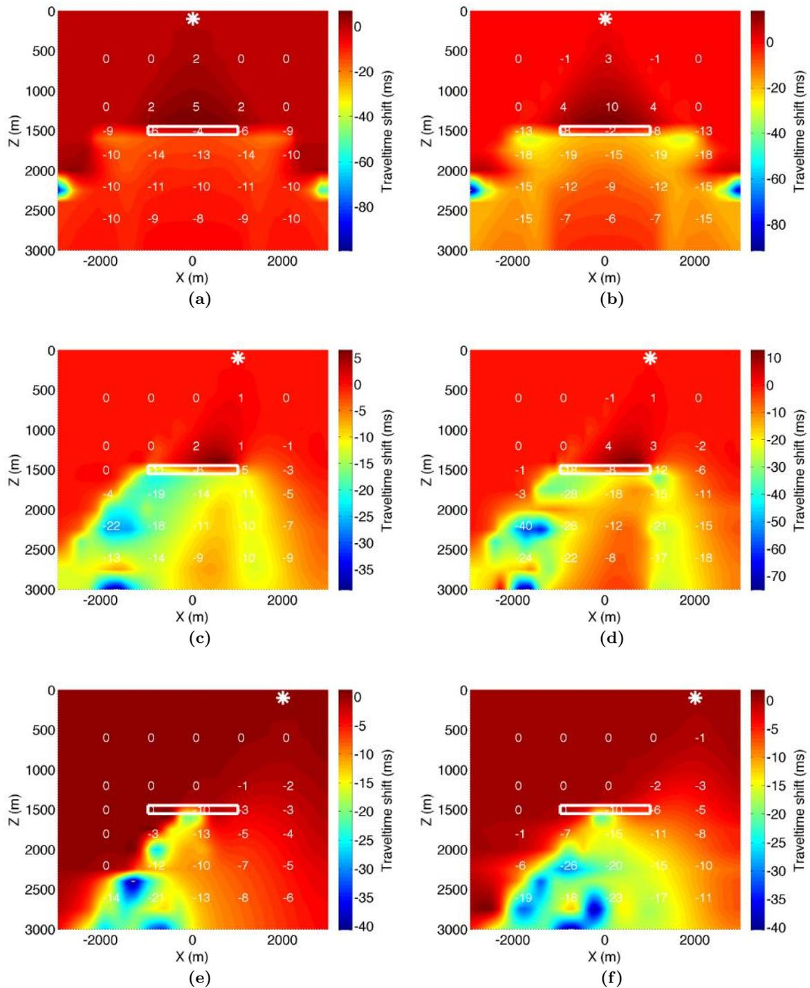
**Figure 4.** P-wave time shifts for the model in Figure 1 (same display as in Figure 2) produced by our modeling package for shot locations of  $X=0$  m (a and b),  $X=1000$  m (c and d), and  $X=2000$  m (e and f). Pore-pressure drops are 5 MPa for the left column, and 20 MPa for the right column. The white rectangle marks the reservoir, while the white asterisk marks the shot location.
