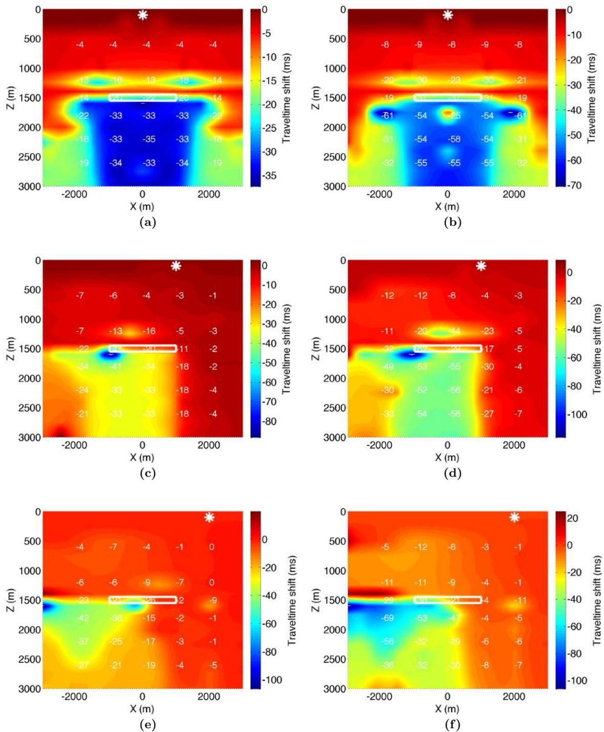
**Figure 6.** S-wave time shifts for the model in Figure 1 (same display as in Figure 4) produced by our modeling package for shot locations of  $X=0$  m (a and b),  $X=1000$  m (c and d), and  $X=2000$  m (e and f). Pore-pressure drops are 5 MPa for the left column, and 20 MPa for the right column.
