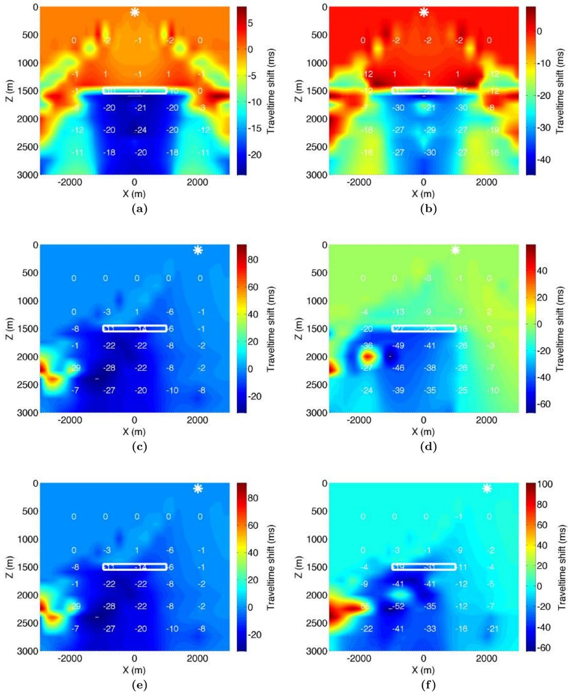
**Figure 5.** PS-wave time shifts for the model in Figure 1 (same display as in Figure 4) produced by our modeling package for shot locations of  $X=0$  m (a and b),  $X=1000$  m (c and d), and  $X=2000$  m (e and f). Pore-pressure drops are 5 MPa for the left column, and 20 MPa for the right column.
