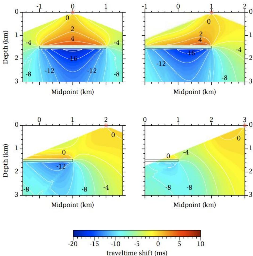
**Figure 2.** P-wave traveltimes shifts computed by ray tracing for the model from Figure 1 (after Fuck et al. (2009)). The asterisk marks the source location at the surface. The time shift (ms) shown at each  $(X,Z)$  point corresponds to the reflection from a horizontal interface at depth  $Z$  recorded at the source-receiver offset  $2(X - X_0)$ , where  $X_0$  is the source coordinate.
