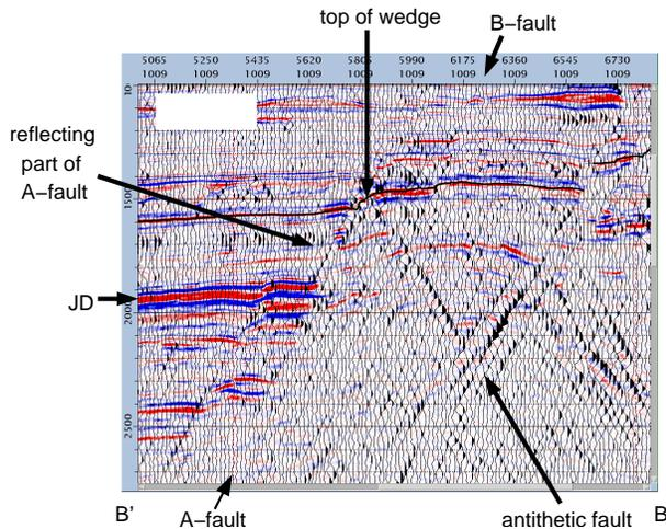
**Figure 7.** An overlay of the time-migrated seismic section along line B-B' with the wiggle-trace slant stack. An antithetic fault exists at this location. The reflecting part of the A-fault corresponds to the part of it between the JD-sand and the top of the wedge formed by the antithetic fault.
