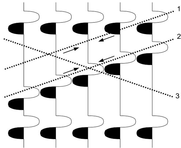
**Figure 4.** The slant stack technique used to accentuate the fault-plane reflections. Stack ‘1’ is zero since it intersects the upper horizontal reflection at an angle. The fault-plane reflection coherently adds into stack ‘2’. We also stacked in the opposite direction ‘3’ to capture any antithetic faults.
