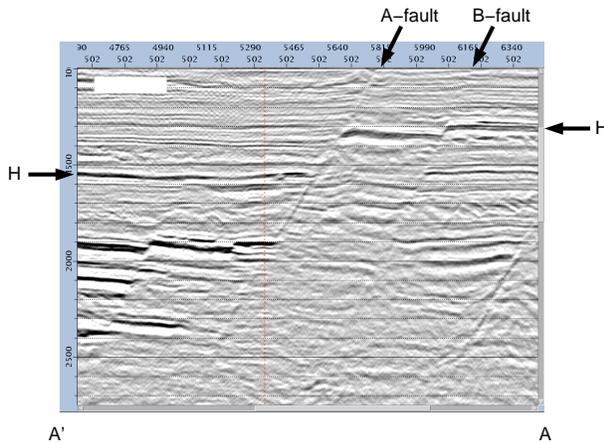
**Figure 3.** A typical fault-plane reflection from the A-fault along the A-A' line. Shown is the post-stack time-migrated image. The H-sand is marked to show the amount of throw across the fault.
