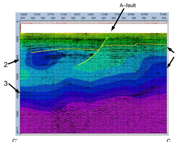
**Figure 2.** Interval velocities along the C-C' line at the South Eugene Island field obtained via a smoothed Dix-type inversion. The velocity increases monotonically with depth at marker '1', but experiences a decrease between markers '2' and '3'. The decrease in velocity with depth indicates that overpressures are present. The general trend of the high velocity pocket at marker '2' correlates with the A-fault.
