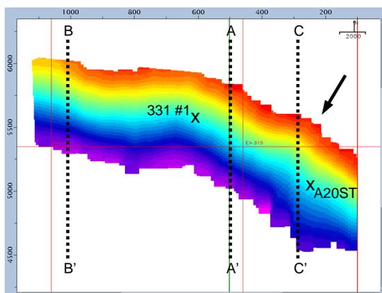
**Figure 1.** Map view of the two-way reflection time from the A-fault. The arrow points in the down-dip direction. Two wells are shown by an X where they intersect the fault-plane. The locations of three seismic lines used in other figures are also shown as dashed lines.
