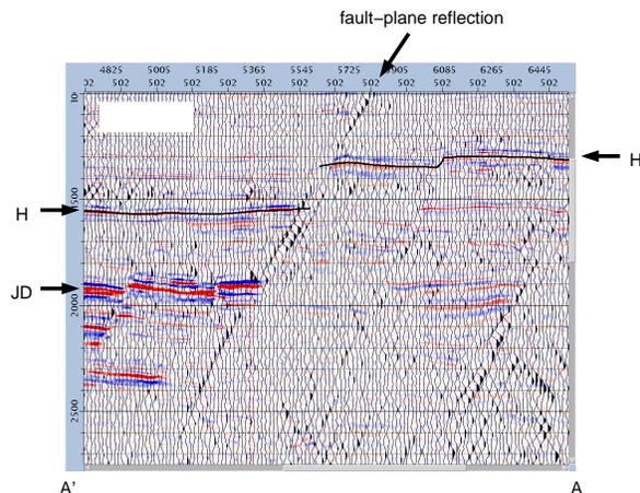
**Figure 5.** Overlay of the time-migrated seismic section from Fig. 1 with the wiggle-trace slant stack. The fault-plane reflection becomes clearer in the slant stack.
