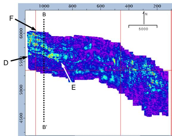
**Figure 6.** Reflection amplitude from the A-fault as a function of position on the fault-plane. The view is the same as in Fig. 1. Stronger amplitudes show up as lighter colors. Points D, E, and F delineate a triangle of higher amplitude on the upper left. Line  $\overline{DE}$  is the intersection of the overpressured JD-sand with the A-fault. Line  $\overline{EF}$  marks the convergence of the A-fault with an antithetic fault. The dashed line B-B' is a seismic section shown in Fig. 7.
