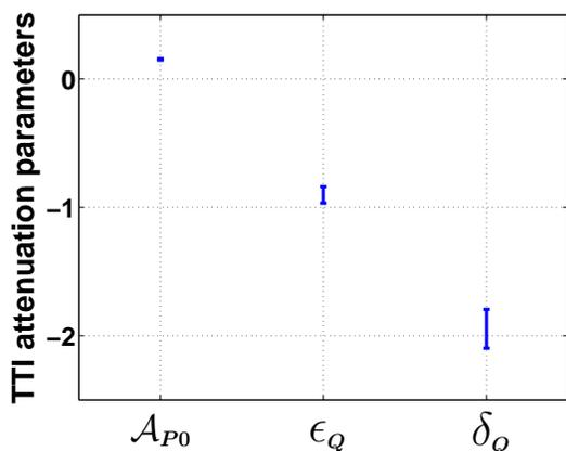
**Figure 8.** Influence of the frequency range used in the spectral-ratio method on the attenuation parameters. The error bars mark the standard deviations in each parameter obtained by applying our algorithm with 50 realizations of the upper and lower bounds of the frequency range. The upper bound was changed randomly between 88 kHz and 132 kHz, and the lower bound between 44 kHz and 66 kHz.
