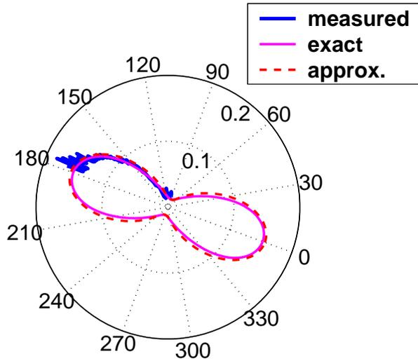
**Figure 6.** Attenuation measurements from Figure 5 (thick solid line) and the best-fit attenuation coefficients obtained using the Christoffel equation (1) (thin grey solid) and the approximation (2) (dashed).
