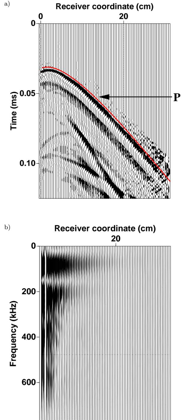
**Figure 2.** (a) Raw transmission data excited by a P-wave transducer, and (b) the amplitude spectrum of the windowed first arrival. The solid line is the P-wave traveltime modeled by Dewangan et al. (2005) using the inverted parameters from Figure 4. The time sampling interval is  $2 \mu\text{s}$ , and the width of the Gaussian window is 40 samples.
