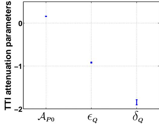
**Figure 7.** Influence of errors in the velocity model on the attenuation parameters. The error bars mark the standard deviations in each parameter obtained by applying our algorithm with 50 realizations of the input TTI velocity parameters. The standard deviations in the TTI parameters are taken from Dewangan et al. (2005).
