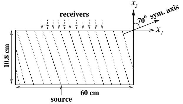
**Figure 1.** Physical model of a TI layer with the symmetry axis tilted at  $70^\circ$  (from Dewangan et al., 2005). The transmitted wavefield is excited by a transducer at the bottom of the model and recorded with a laser vibrometer.
