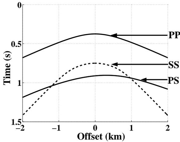
**Figure 7.** CMP gathers of reflected waves for the model in Figure 2 computed by anisotropic ray tracing. The PS-wave is converted at the dipping interface, while the PP- and SS-waves are reflected from the bottom of the overburden.
