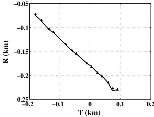
**Figure 8.** Source and receiver coordinates of the PS-wave at the top of the target layer obtained for the model in Figure 2. Here and in Figure 9 the triangles are the output of the layer-stripping algorithm applied to the data in Figure 7; the solid line marks the results of ray tracing.
