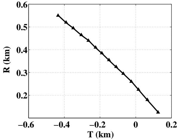
**Figure 4.** Source and receiver coordinates at the top of the target layer obtained for the model in Figure 2 for a range of surface points  $[x^{(3)}, x^{(4)}]$ . Here and in Figure 5 the triangles are the output of the layer-stripping algorithm; the solid line marks the results of ray tracing.
