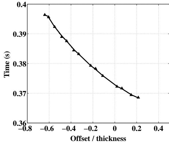
**Figure 9.** Interval PS-wave traveltimes in the target layer as a function of offset for the source/receiver pairs from Figure 8.
