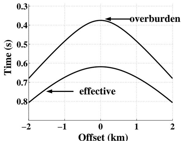
**Figure 3.** CMP gathers of the PP-wave reflections from the bottom of the second layer (marked “overburden”) and the dipping reflector (“effective”) for the model in Figure 2. The traveltimes were generated by an anisotropic ray-tracing code.
