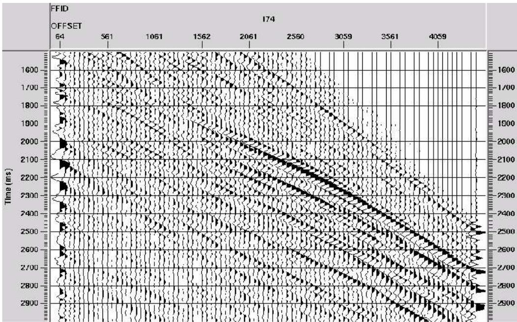
Figure 2. Gather from Figure 1 after application of F-K filtering designed to attenuate overburden noise. The target event marked in Figure 1 is clearly visible between 1500 m and 4500 m.
