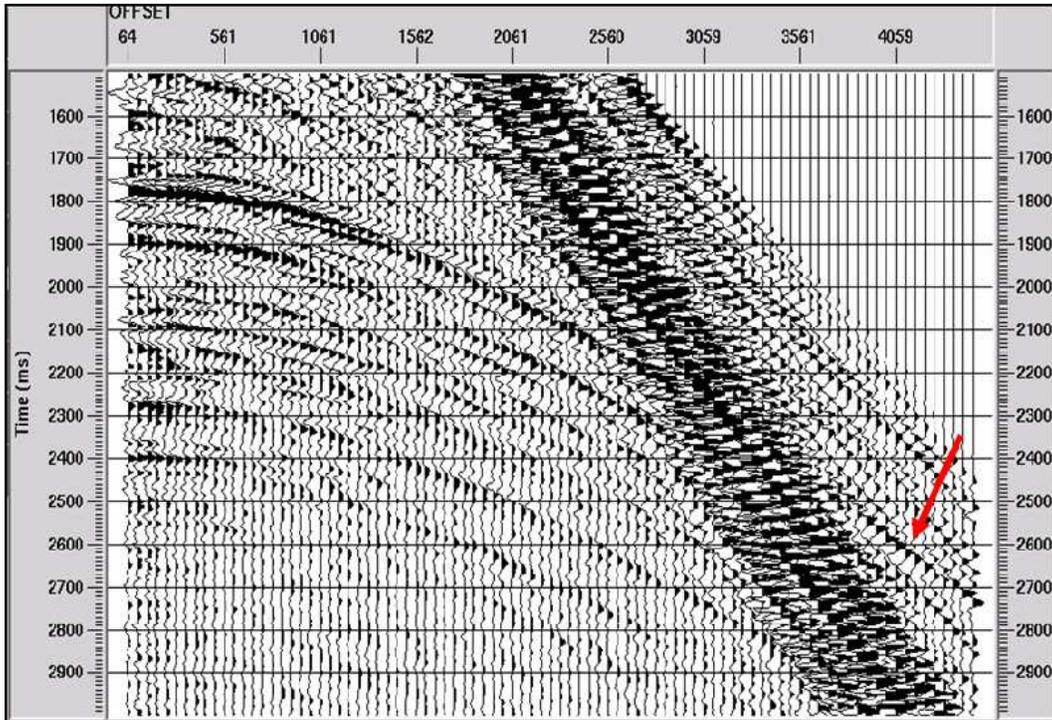
Figure 1. Common-receiver field gather of the vertical displacement component. The arrow marks a reflection from the top of a high-velocity layer.
