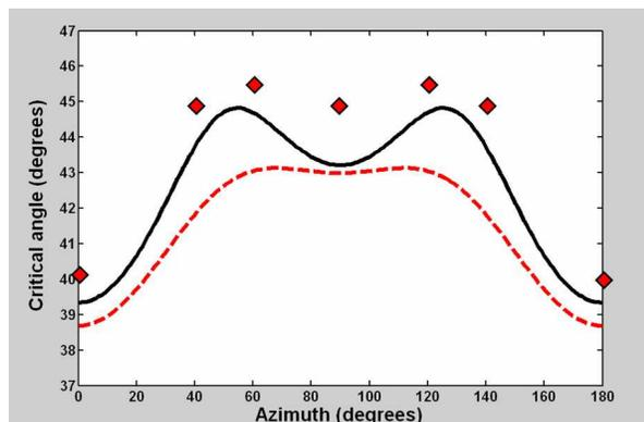
**Figure 7.** Variation of the critical angle with azimuth for the model from Figure 5. The diamonds mark the critical angle estimated from the reflectivity modeling, the solid line is the exact critical angle, and the dashed line is computed from three weak-anisotropy approximation 12.
