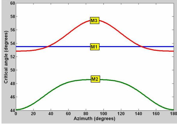
**Figure 4.** Critical angle of P-waves computed as a function of azimuth from equation 12. The parameters of models M1, M2, and M3 are listed in Table 1. The azimuthal anisotropy of the top (incidence) layer in models M2 and M3 causes a noticeable variation of the critical angle with azimuth.
