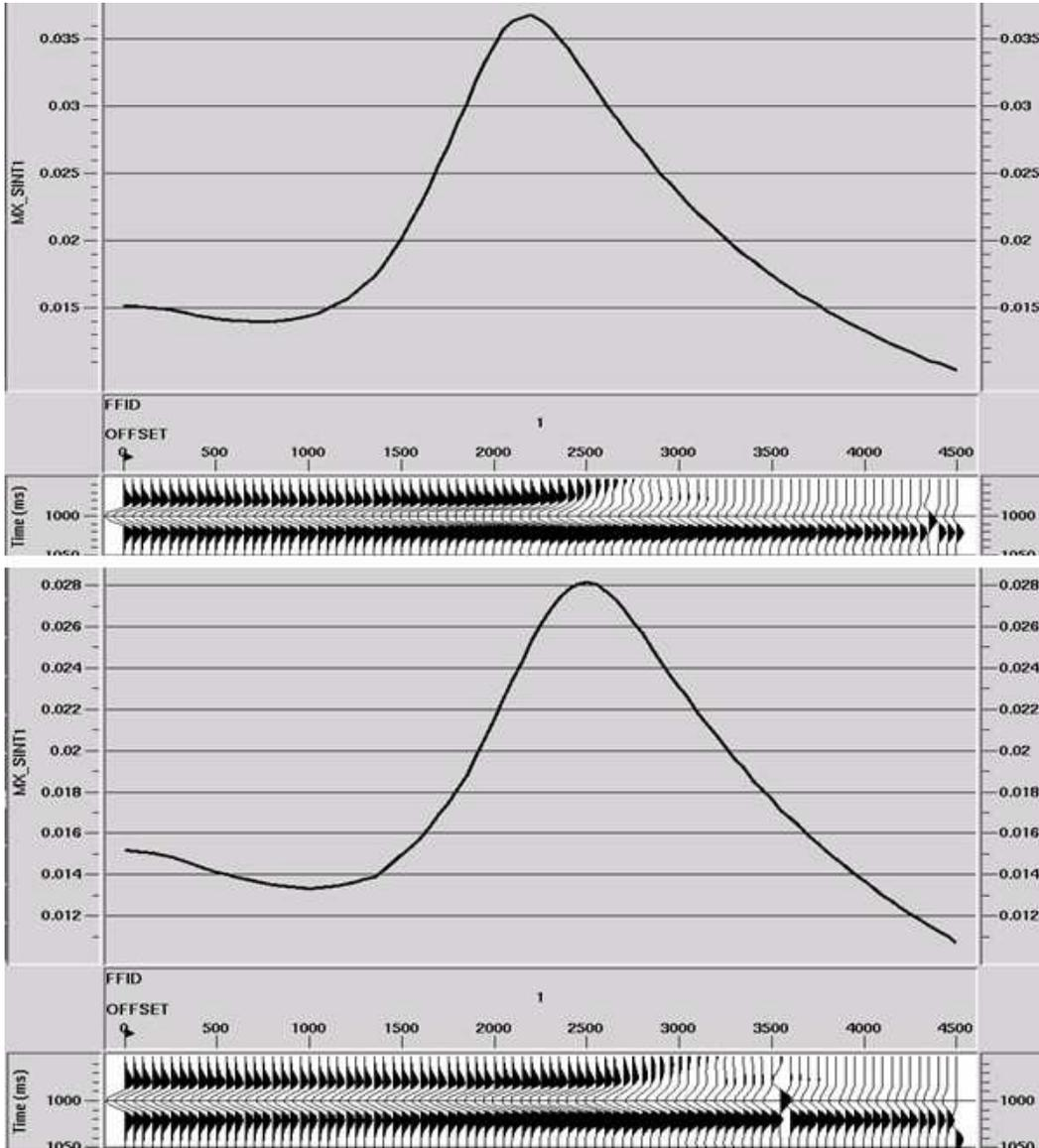
**Figure 6.** Amplitude of the reflected PP-wave from Figure 5 as a function of offset for the azimuths  $\phi = 0^\circ$  (top) and  $\phi = 40^\circ$  (bottom). The offset of the amplitude maximum is 2200 m for  $\phi = 0^\circ$  and 2450 m for  $\phi = 40^\circ$ .
