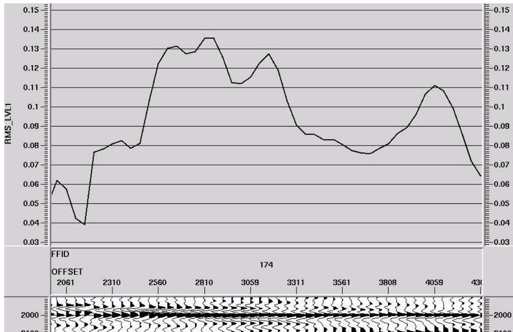
**Figure 3.** Estimated RMS amplitude of the target event from Figures 1 and 2 computed in a 50 ms window after F-K filtering. The offset of the fastest amplitude increase, which we interpret as corresponding to the critical-angle reflection, is near the 4 km mark. The windowed section on the bottom shows the flattened target event.
